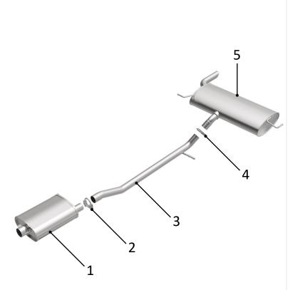
(Carefully read all instructions before installation) Disconnect the vehicle's battery before removal of the OEM exhaust system. This will prevent electrical accidents and will reset the computer if it applies to the vehicle. Remove existing exhaust system from the vehicle. Only remove parts that will be replaced. Clean existing flange with a wire brush to ensure proper sealing.
